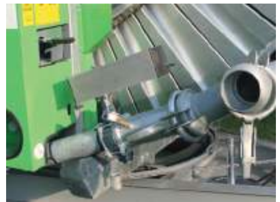
Shut-off valve Optimum safety thanks to automatic shut-off of the system in case of over- or underpressure
