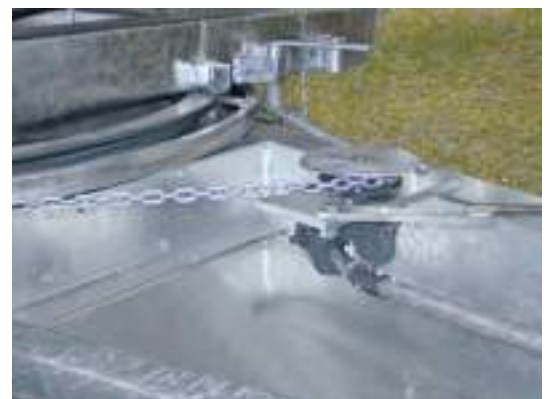
Option: swivel aid – mechanical or hydraulic For easy swivelling of the reel even on uneven grounds
