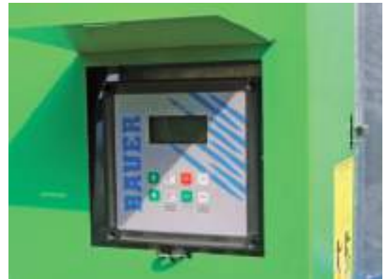
Ecostar 4000 S Irrigation computer provides exact demand of required precipitation rate
